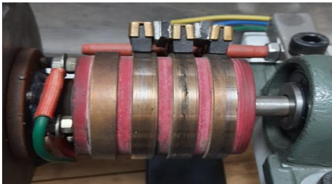
Fig.3 Three phase commutator with carbon brush.
