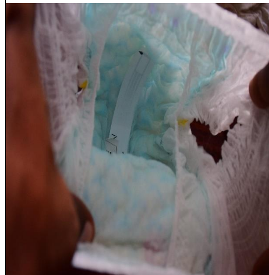
The internal placement of passive wireless sensor in the diaper
