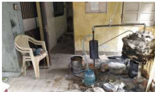
Figure 3 Plastic waste digestion process setup with the first prototype
