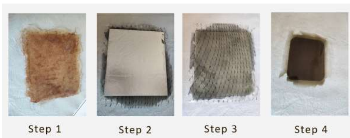
PCB made of shellac modified resins
