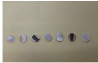
electrode patterning on the substrate using thermal evaporation.
